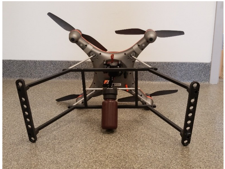
Figure 1. Aircraft with water sampling bottle attachment shown
