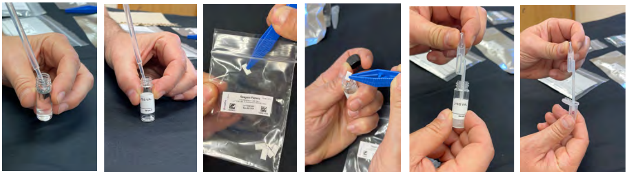
Figure 3: various steps involved in sample preparation for ABRAXIS test kit
