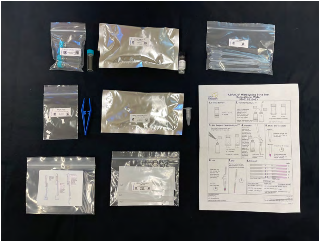
Figure 2: Components included in ABRAXIS test kit.
