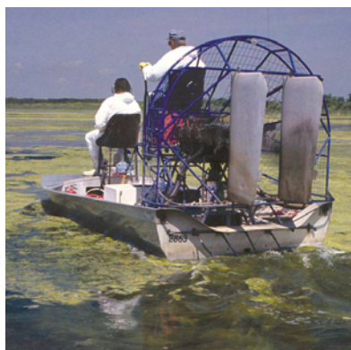
Figure 6. An application of aquatic herbicide using an airboat with trailing hoses for treating hydrilla. Note: Filamentous algae is on the water's surface and hydrilla is below.
