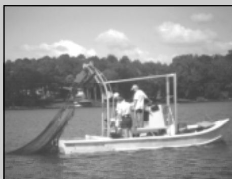
Top: Electrofishing boats are rigged with special equipment that sends an electric current into the water, temporarily stunning fish. The fish are netted, counted, measured, and then released back into the water.
