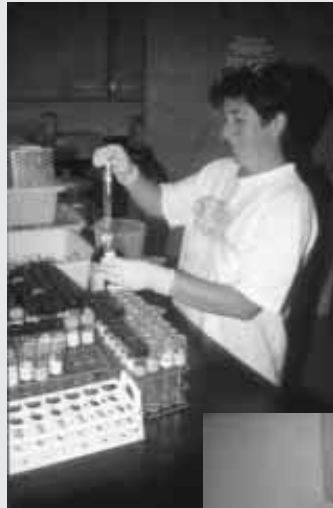
Left: Kelly Schulz adds a solution of potassium persulfate to test tubes containing lake sample water. The potassium persulfate helps to digest or "free up" nutrients (phosphorus and nitrogen) in the water so they can be measured.
