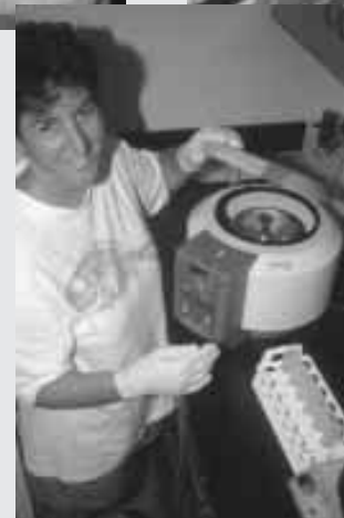
Left: Kelly Schulz places test tubes containing phosphorus samples into the centrifuge, a device that will spin the test tubes at high speeds, forcing sediments to the bottom. Once the samples have been 'centrifuged,' they are ready to be analyzed for phosphorus values on the spectrophotometer.
