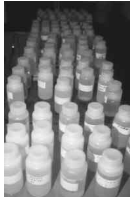
Water sample bottles cover the countertops as they defrost in the water chemistry laboratory. Each month, the laboratory conducts over 5400 separate analyses for LAKEWATCH: 600 lakes X 3 samples per lake X 3 parameters (nitrogen, phosphorus, chlorophyll).
