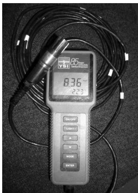
A digital DO meter used by LAKEWATCH.
