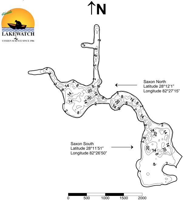
Florida LAKEWATCH personnel created this map using differentially corrected global positioning equipment (GPS). Data were collected August 8, 2000. Scale and map contours are in feet and were generated using kriging technique in Surfer® software package (Golden CO). On this date, the lake surface area was calculated at 68 acres (28 hectares). This is only an approximate bathymetric map and should not be used for navigation.<sup>1</sup>
