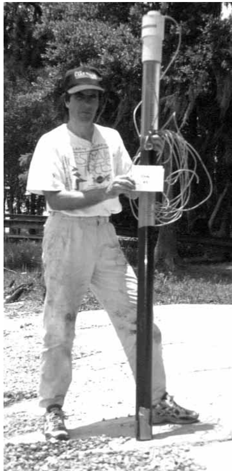
Tom Whitmore, a paleolimnologist, is shown here with a sediment corer. Tom uses lake sediments to determine what types of algal communities were present in Florida lakes in pre-LAKEWATCH days.
