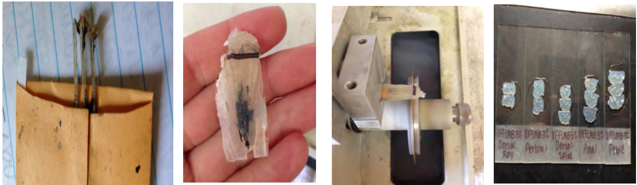
Figure 2. A) Dorsal rays 3-5 excised and cleaned, prepped for the drying box, B) dorsal spines III-V imbedded in two-part epoxy, C) sectioning a fin structure with the low speed saw, and D) cross-sections (~0.7-1.4 mm) of several fin structures permanently mounted to slides.
