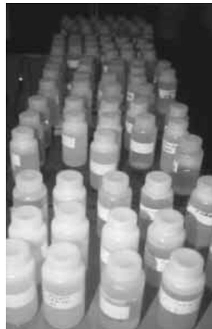
*Water sample bottles cover the countertops as they defrost in the water chemistry laboratory. Each month, the laboratory conducts over 5400 separate analyses for LAKEWATCH: 600 lakes X 3 samples per lake X 3 parameters (nitrogen, phosphorus, chlorophyll).*
